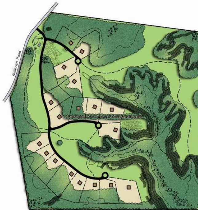
Figure 1. The Growing Greener model land use regulations first delineate open space areas based on local protection priorities before development areas are designed.
