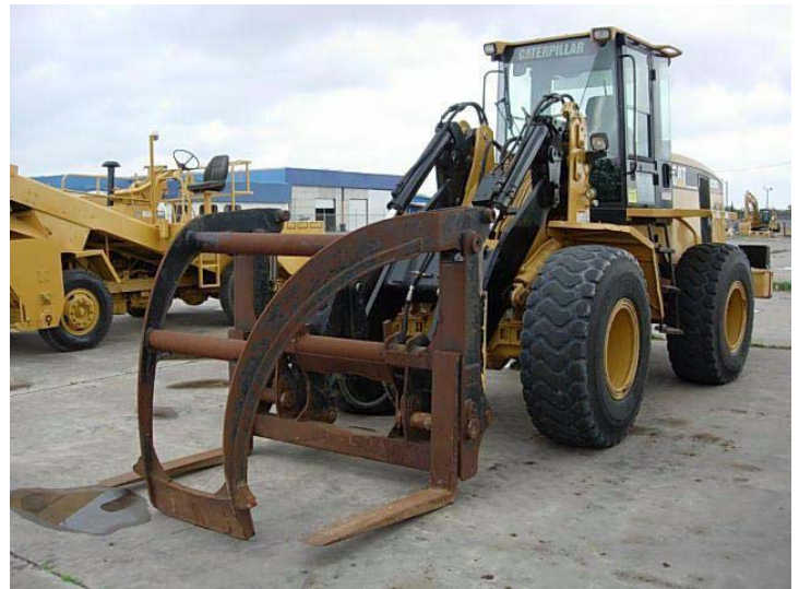
Illustration 2: Standard Rubber Tire Loader placement) up to 4 psi might be allowable.
