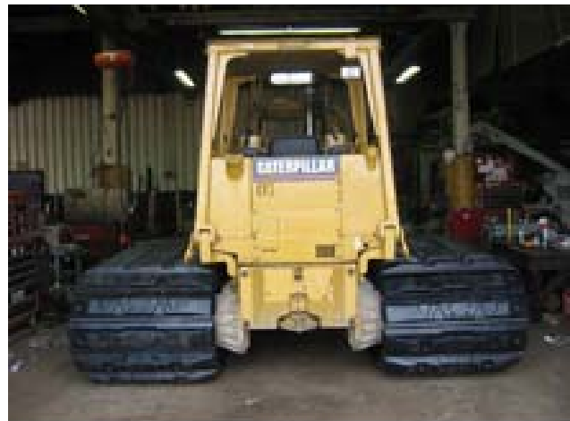
Nyrin Track Pads on CAT 939C Loader
